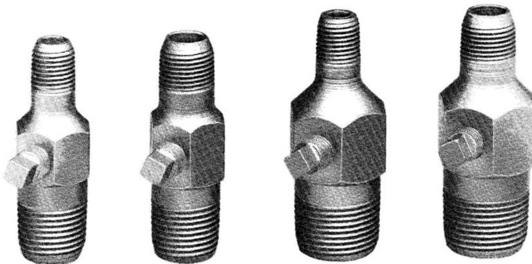
Eclipse Flame Scanner Adapters permit quick, easy installation of ultraviolet flame scanners to burner connections of a different pipe size. Made from heavy steel, these adapters are supplied with a 1/8" N.P.T. tap to permit connection of a purge air line, if required.
